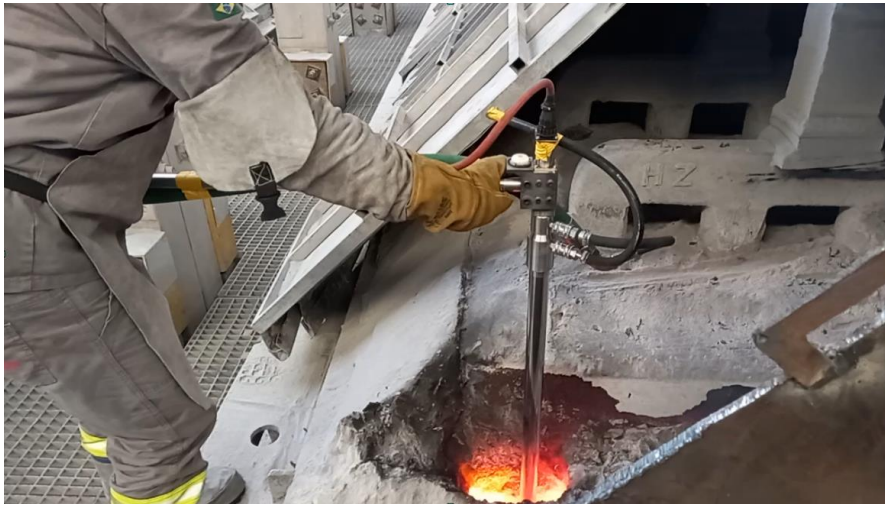
Figure 9. Magnetic field measurement in the operating cell.
